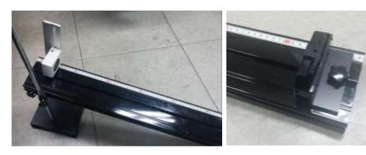
2. Calculate the height h of the rail for angles  $\theta$  of 5°, 10°, and 15° using the length L of the rail and trigonometric functions or a 3-axis accelerometer.
