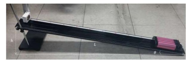
3. Adjust the height  $\hbar$  to fix the rail at an angle  $\theta$  of 5°.
